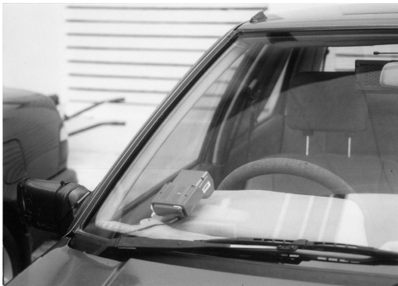
Figure 5 The IU is normally located in the lower right-hand corner of the windscreen
