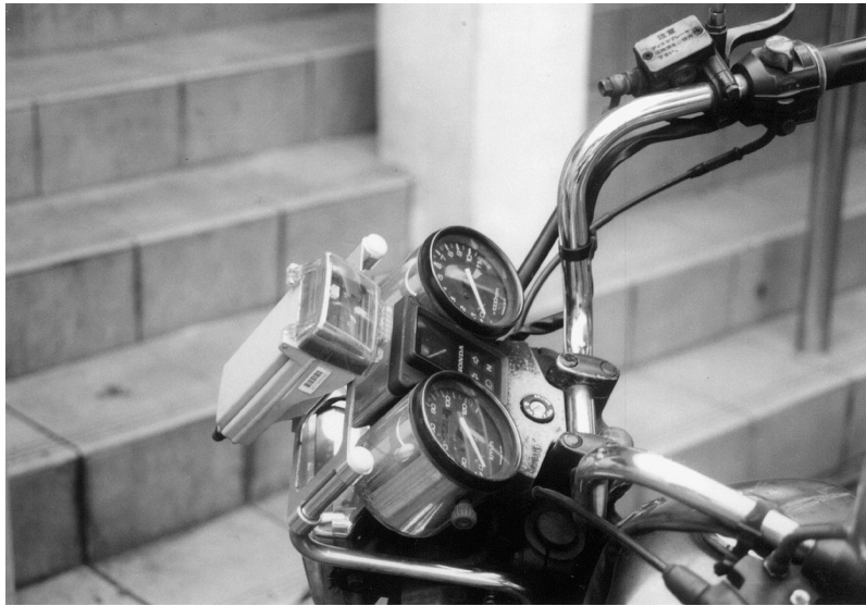
Figure 6 The motorcycle IU has a protective covering to prevent rainwater seepage
